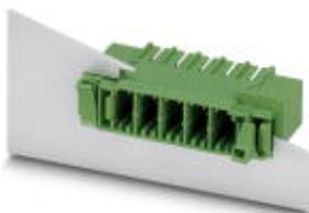
Feed-through header, nominal current: 41 A, rated voltage (III/2): 630 V, nominal cross section: 6 mm<sup>2</sup>, number of positions: 11, pitch: 7.62 mm, color: green, contact surface: Tin, mounting: Wave soldering, pin layout: Linear pinning, solder pin [P]: 4.9 mm
