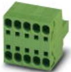
PCB connector, nominal current: 41 A, rated voltage (III/2): 1000 V, nominal cross section: 6 mm<sup>2</sup>, number of positions: 11, pitch: 7.62 mm, connection method: Push-in spring connection, color: green, contact surface: Tin
