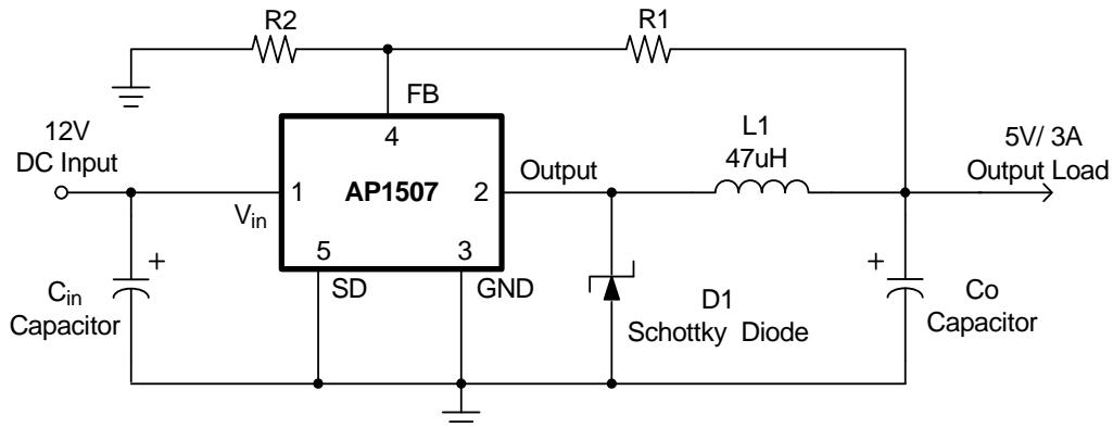
$$V_{OUT} = V_{FB} \times \left(1 + \frac{R1}{R2}\right)$$
