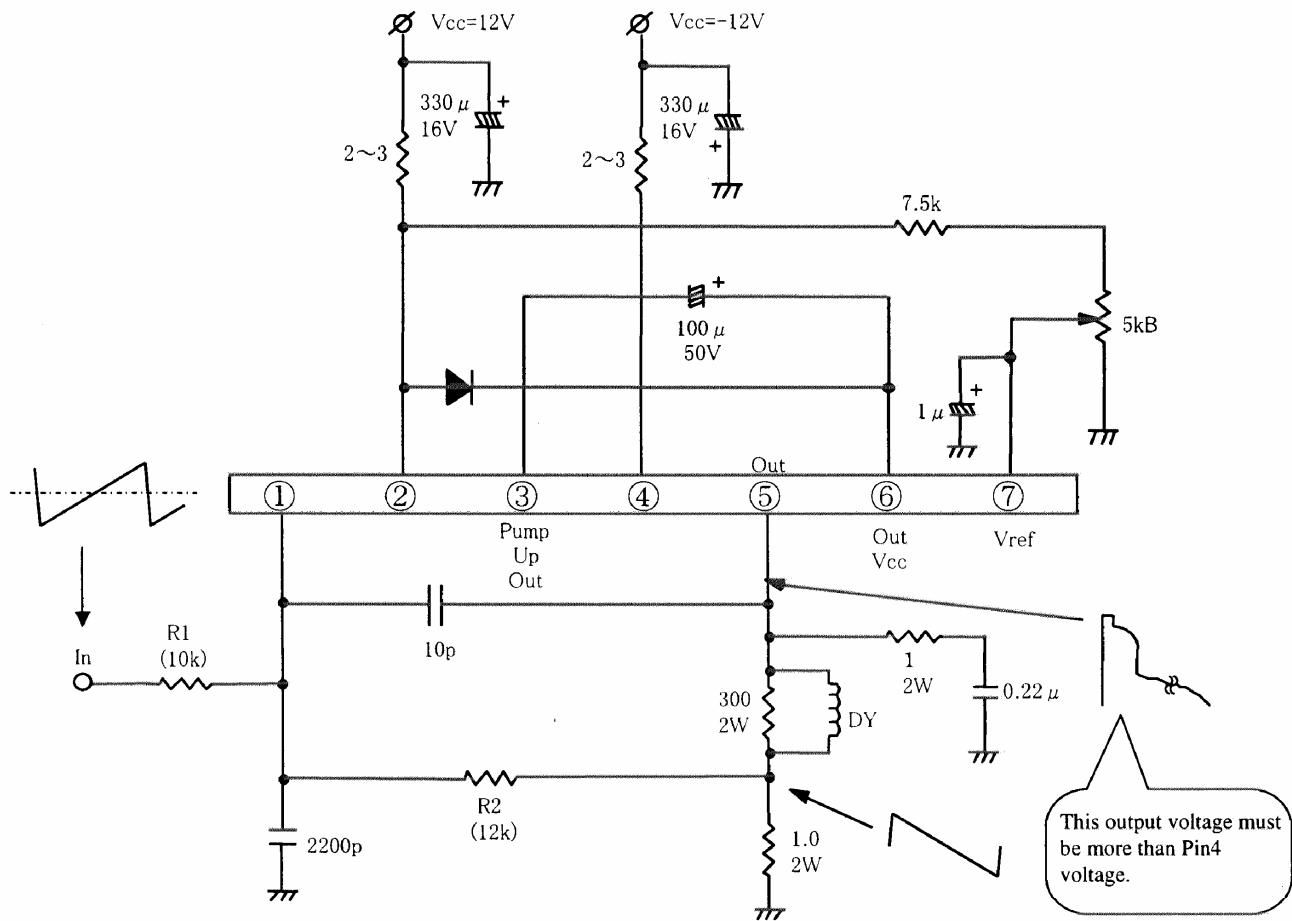
In order to get required gain, it is necessary to adjust the R1 and R2.
