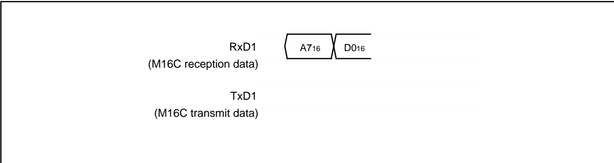
Figure 5.6.22. Timing for erasing all blocks
