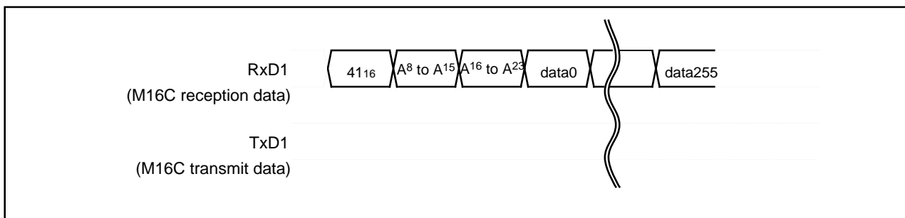
Figure 5.6.20. Timing for the page program
