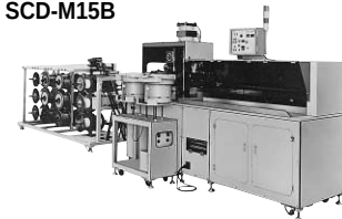
Auto. ID machines for shielded wires SCD-M15B
