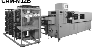
Auto. ID machines for multi-harnesses CAM-M12B
