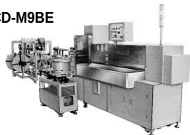
Auto. ID machines for 2.5 mm (.098") & 2.0 mm (.079") pitch jumper wires
