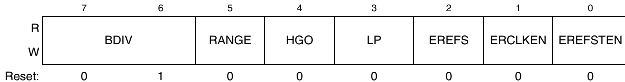
Figure 8-4. ICS Control Register 2 (ICSC2)
