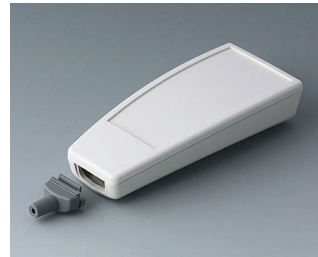
A9067137 SMART-CASE L, Vers. IV ABS (UL 94 HB) off-white RAL 9002 5.51"x2.47"x1.20" IP 65 opt., IP 40
