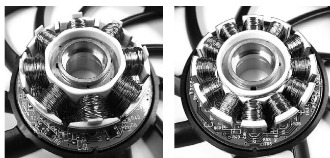
Current model (9GV type) New model Fig. 6: Motors of new model and current model
