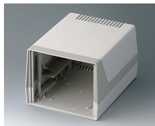
A9917847 LUX CASE 230, Vers. II ABS (UL 94 HB) off-white RAL 9002 6.81"x9.06"x5.35"
