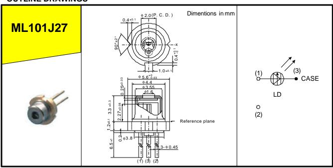
There is no model with a monitor photo diode in ML1XX27 series.
