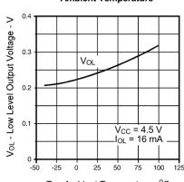
T<sub>A</sub> - Ambient Temperature - °C
