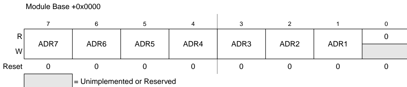
Figure 10-3. IIC Bus Address Register (IBAD)
