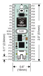
The PropStick USB is suitable for all new Propeller-based designs, whether prototype or production. PropStick USB mounting possibilities include breadboard, perfboard with wire-wrap, or in a 600 mil 40-pin socket soldered to a PCB.
