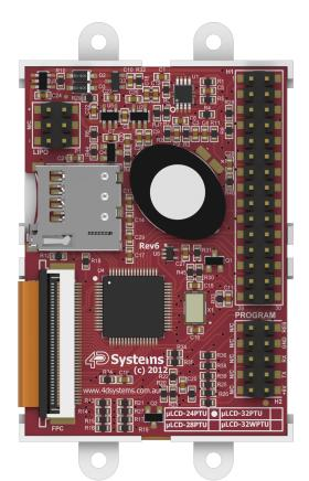
The  $\mu$ LCD-24PTU has a **2.4"** TFT LCD display at the forefront of the design that showcases the power and capabilities of the PICASO processor. Combining a resolution of **240x320** pixels with **65K** True to Life colours, this module is perfect for animations, slideshows and other multimedia presentations.
