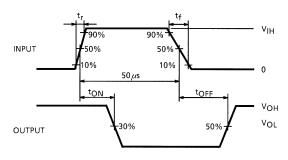
Note 1: Pulse Width 50  $\mu$ s, Duty Cycle 10% Output Impedance 50  $\Omega$ ,  $t_f \le 5$  ns,  $t_f \le 10$  ns
