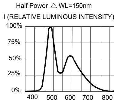
FIG.4 RELATIVE LUMINOUS INTENSITY VS.
