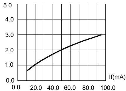
FIG.3 RELATIVE LUMINOUS INTENSITY VS.
