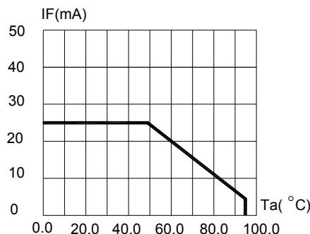
FIG.5 MAXIMUM FORWARD DC CURRENT VS.
