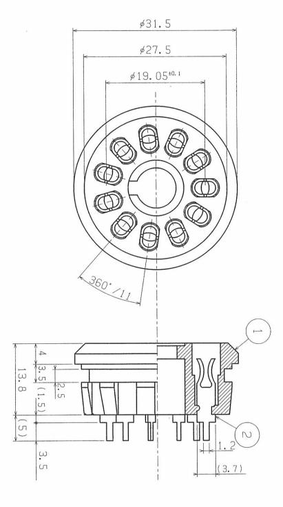
SPECIFICATION: A)Contact Resistance:Less than 10 m-ohm.
