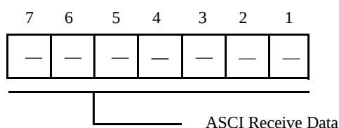
Figure 31. ASCII Receive Register Channel 1R
