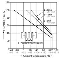
3. On resistance vs. ambient temperature characteristics
