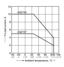
2. Load current vs. ambient temperature characteristics in adjacent mounting Sample: All types
