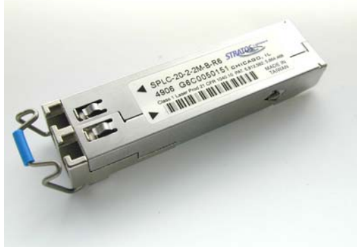
Figure 12-3 Stratos Single-Mode Intermediate-Reach SFP — Mfg. Part #: SPLC-20-2-2M-B-R6 — Harris Part #: ATM-OPT-SM
