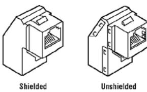
Two Category 5 feed-thru modular couplers are available for mating EIA568A or B Category 5 connections. Couplers come in shielded and unshielded version, the unique offset design maintains Category 5 performance and limits depth to only 1.25". Designed to mate with keystone style holes. Color: Black.
