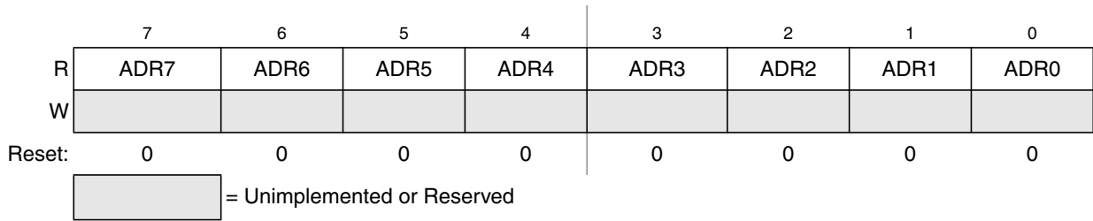
Figure 14-7. Data Result Low Register (ADC1RL)
