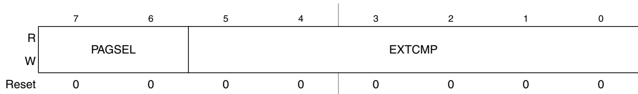
Figure 18-15. Debug Comparator A Extended Register (DBGCAx)
