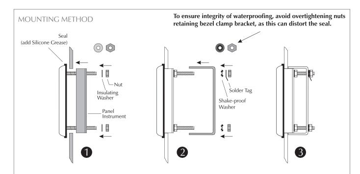
Notes: On some panel instruments it may be easier to configure links and calibrate the product prior to fitting the instrument and BEZ 700-IP into the panel. Always observe safety warnings on the Panel Instrument datasheet. Do not allow connections to touch the metal bezel, as this may adversely affect product safety or stop the panel instrument from functioning correctly.
