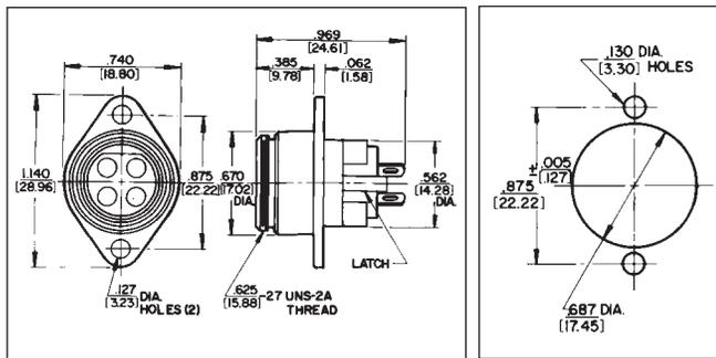
Flange mounted; 2 through 5 pins (male) or 2 through 5 contacts (female). Also 2-, 3- and 4-contact inserts with 2 shunted (N.C.) contacts.
