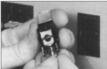
Remove escutcheon and lever assembly. (see "MOUNTING" above) For relamping, pull lamp out of retainer with finger-tip. Replace lamp.
