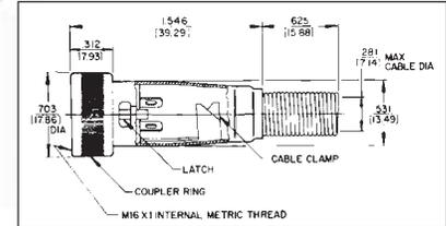
**CB-3M** 3-pin male receptacle. Housing keys insert of mating plug; bushing with external M16x1 metric thread mates with coupling ring on plug. Cup-type terminals accept wires up to #16 AWG. Mounts in .64" (16.26 mm) diameter hole from front of panels up to .125" (3.18 mm) thick, using washer and locknut supplied. Can also be "D"-hole mounted for non-turn mounting (see drawing). Pin diameter is .093".
