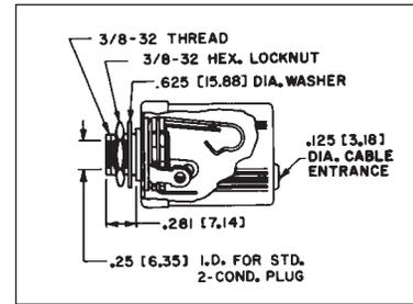
Shield is assembled as part of the jack; cover "snaps" into place. Shield is designed for Hi Z circuits. Mounting is through a 3/8" diameter hole in chassis/panel up to .156" thick with hex nut and flat washer (supplied). On special order, jacks with .21 inch inside diameter bushing are available.
