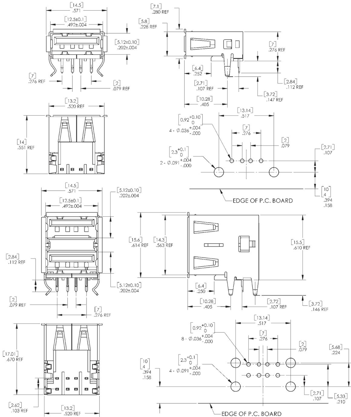
DIMENSIONS ARE FOR REFERENCE ONLY  $\frac{\text{Inch}}{\text{(mm)}}$
