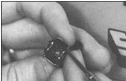
For color filters, use fingernails or small screwdriver to remove. Gently lift (don't pry) up under edge of filter until it "pops" out.
