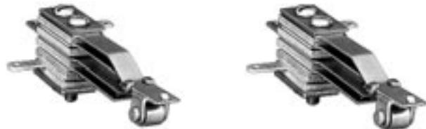
Thousands of switching combinations are possible with slightly smaller parts. Mounting centers are .250" (6.35 mm) (minimum) with .188" (4.78 mm) wide parts. Practical spring length is 2.125" (53.98 mm) (maximum). Contact Switchcraft for selection of contacts and ratings.
