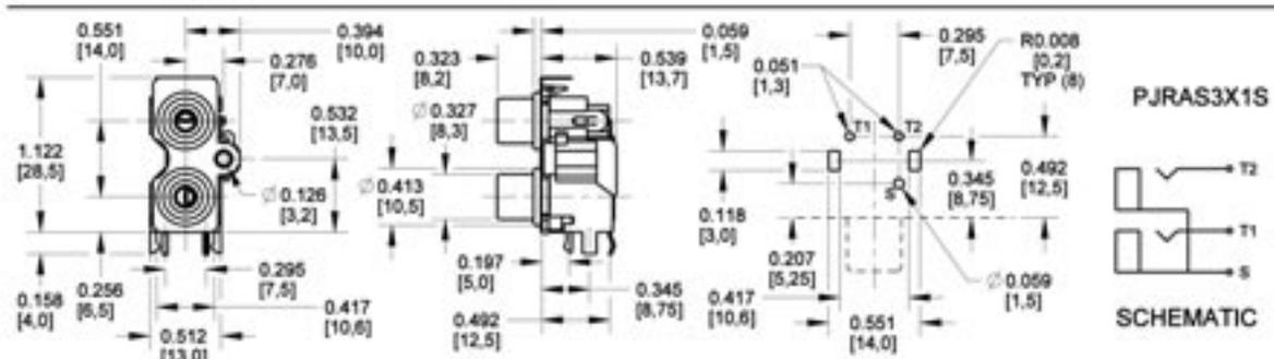
DIMENSIONS ARE FOR REFERENCE ONLY  $\frac{\text{Inch}}{\text{mm}}$
