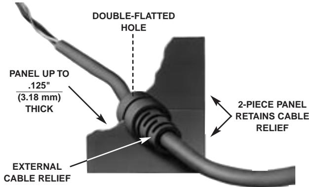
CUTAWAY VIEW OF STYLE ST303
