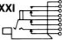
Tip closed; ring closed circuits. Isolated switching—"break" before "make" circuit.
