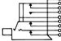
Double closed circuit. Isolated switching—One "make" and one "break" circuit.
