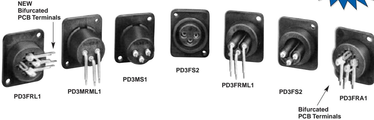
Switchcraft offers the PD Series (plastic panel mount) audio connectors with a wide variety of 3-pin/contact, male and female types and many terminals for combined PC/panel mount. Female types offer larger contact area for higher ratings and longer life. Panel mounting may be at users option, either front or rear. New PD series connectors mate with Switchcraft Q-G and other compatible types.
