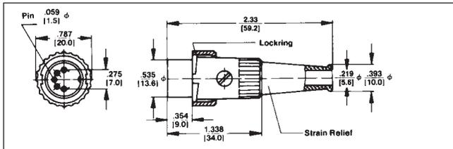
**Type 05CL5M – typical** Male plug with ground key-rib. Unique 30° turn locking securely fastens two halves of connector. Mates with lock flange female connectors and receptacles. Insert screw holds insert assembly in shell and also retains locking on shell. Flexible black strain relief with 7/32" diameter cable entry. Heavy duty clamp.
