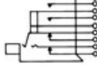
Double closed circuit. Isolated switching—Two "make" circuits.
