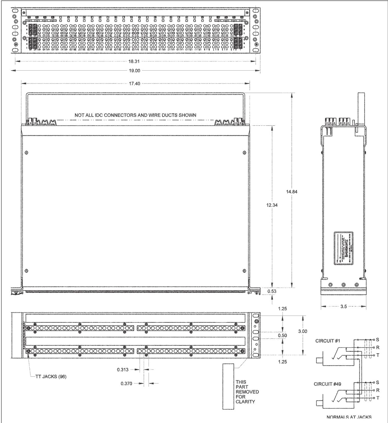
DIMENSIONS ARE FOR REFERENCE ONLY  $\frac{\text{Inch}}{(\text{mm})}$
