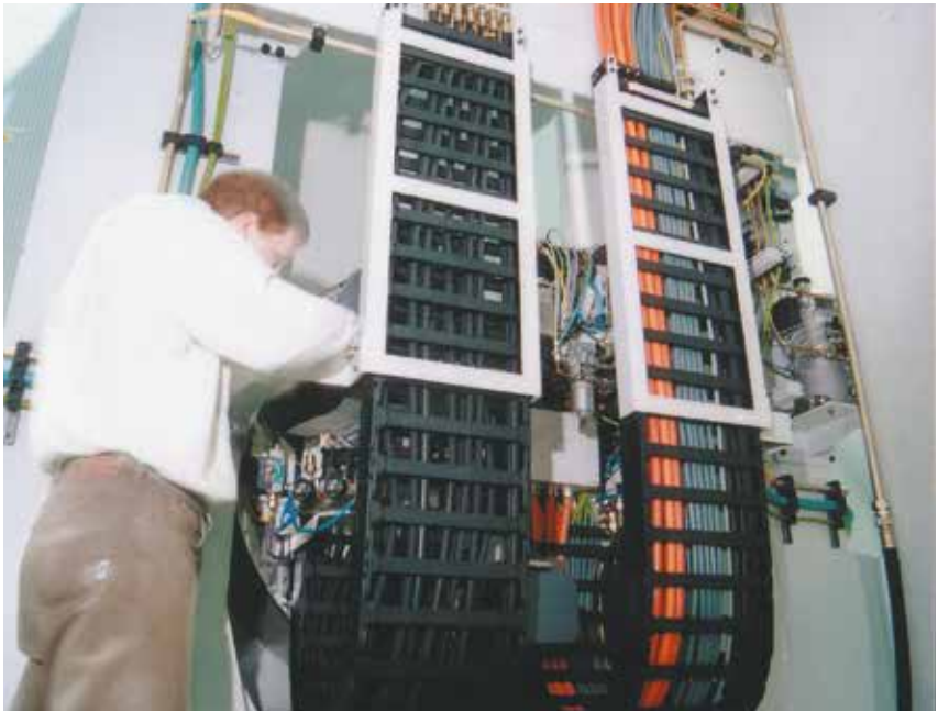
Modular design, easy to retrofit: igus® E4 E-Chain® and Chainflex® cables.
