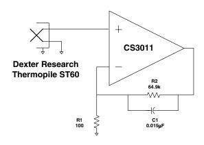
Thermopile Amplifier with a Gain of 650 V/V
