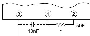
Adjust/comp (pin 3) may be driven by external circuitry referenced to pin 2 (-output) if desired. Grounding pin 3 causes voltage to increase (25% typically) while driving pin 3 above 1.3 V causes output voltage to decrease. Pin 3 may be driven through 10K $\Omega$  or more if connection of the comp function is also required.
