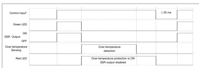
\*After over-temperature condition is removed, SSR can be reset by switching OFF the control input for more than 20 ms and switching back ON: this will switch ON the SSR output
