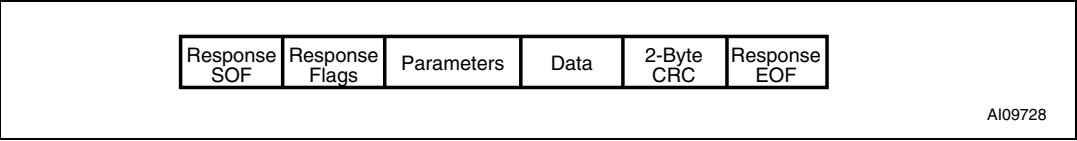
Figure 17. LRI64 response frame format
