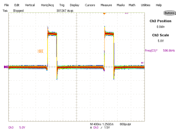
Fig. 11: Inductor node at 12A load Ch 3 :LX
