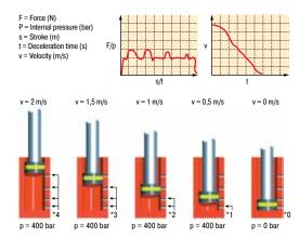
\* The load velocity reduces continuously as you travel through the stroke due to the reduction in the number of metering orifices (\*) in action. The internal pressure remains essentially constant and thus the Force vs. stroke curve remains linear.
