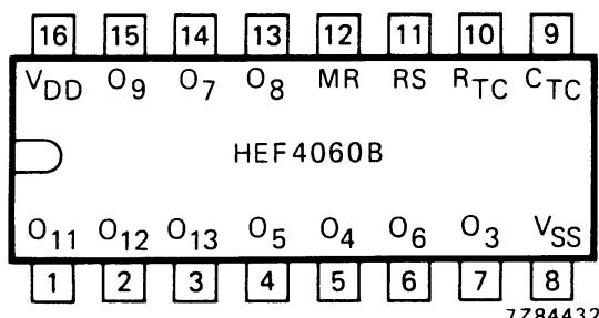
Fig.2 Pinning diagram.
