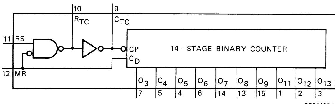
Fig.1 Functional diagram.
