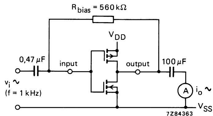
Fig.6 Test set-up for measuring forward transconductance  $g_{fs} = di_o/dv_i$  at  $v_o$  is constant (see also graph Fig.7);
