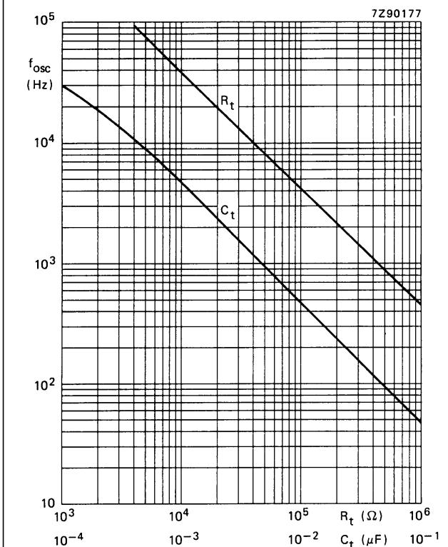
$C_t$  curve at  $R_t = 100$  k $\Omega$ ;  $R_2 = 470$  k $\Omega$ .
