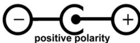
Figure 2-1. Power Supply Barrel Connector (J2) Polarity
