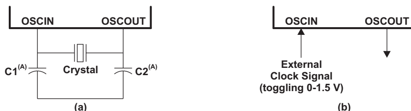
Figure 5-5. Recommended Crystal/Clock Connection
