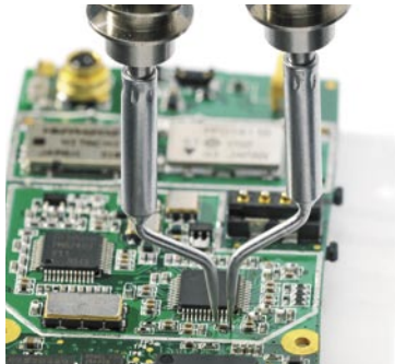
Special Chip Tool tips for 0201 rework.
