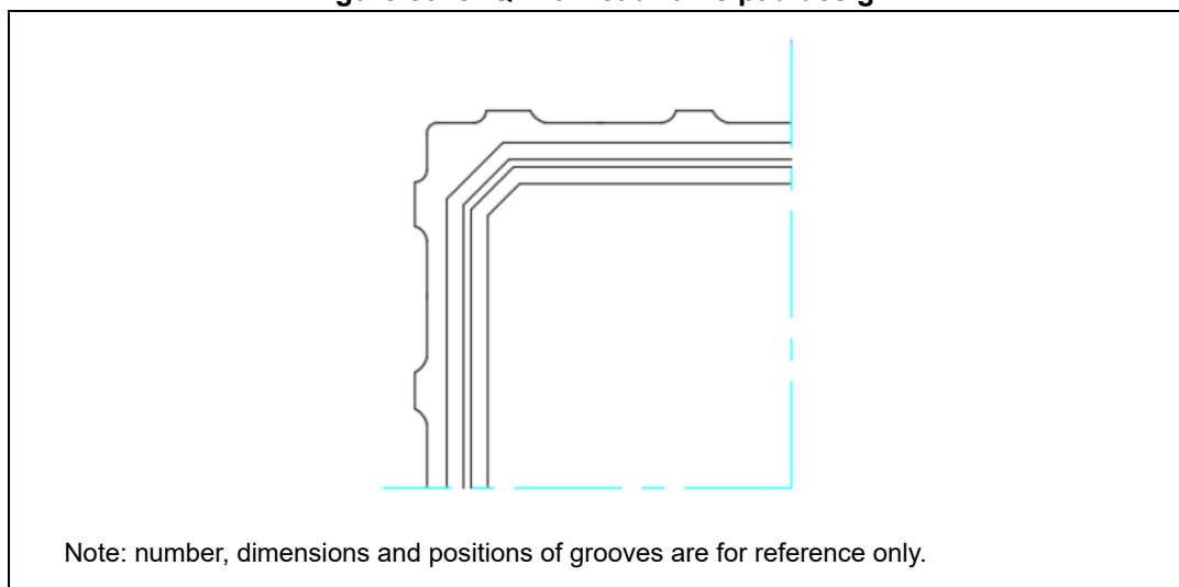
Figure 50. eTQFP64 leadframe pad design
