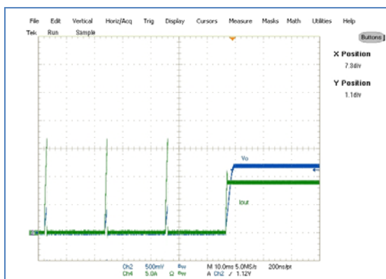
Figure 35: Short Circuit Recovery, Ch2: V_{out} , Ch4: I_{out} (5A/Div)
