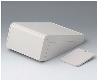
B4056207 UNITEC M, 0.02/0.02 ABS (UL 94 HB) off-white RAL 9002 5.83"x8.27"x3.15" IP 40
