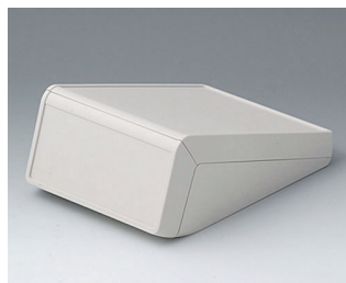
B4056117 UNITEC M, 0.06/0.06 ABS (UL 94 HB) off-white RAL 9002 5.83"x8.27"x3.15" IP 40
