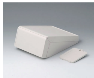
B4054237 UNITEC S, 0.02/0.06 ABS (UL 94 HB) off-white RAL 9002 4.92"x6.97"x2.72" IP 40
