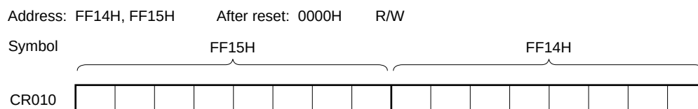
★ Figure 6-4. Format of 16-Bit Timer Capture/Compare Register 010 (CR010)
